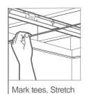
string across the room at each main-tee location. Stretch one string perpendicular to mark the rst row of 6 in. below the string cross tees. (Main tees have pre-punched line.Bend each hanger slots that will align the wire to a 90-degree angle 3/4 in. above the remaining cross tees.)
